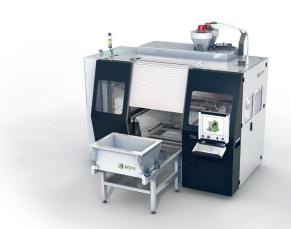
The S-Print combines a compact structure with an extremly versatile range of applications. With the flexibility to select any binder system available at ExOne, S-Print sand molds can be made to accommodate a variety of casting materials for rapid product development and short run production.
